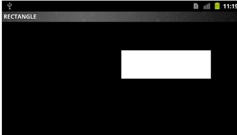
Figure 3-14. Rendering rectangle using triangle primitives
