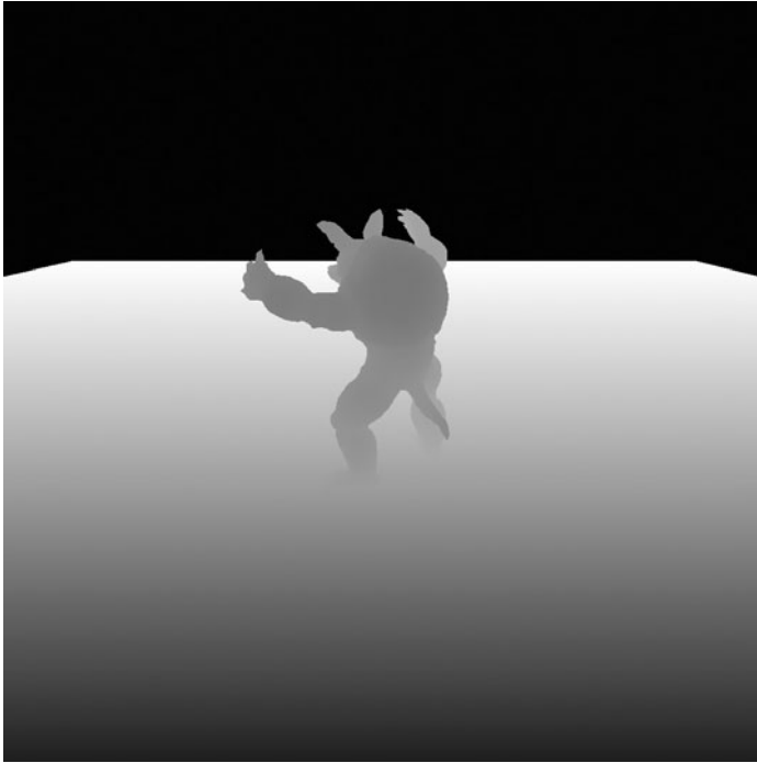
Figure 7.10 Depth rendering (Depths are rendered from the light's position. Within rendered objects, closer points have smaller depths and show up darker.)
