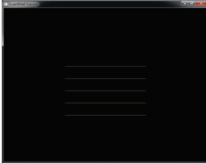
Figure 8.7: Isoline tessellation example
