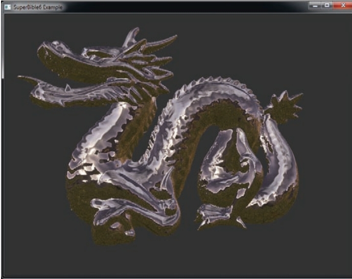
Figure 12.13: Rendering result of equirectangular environment map
